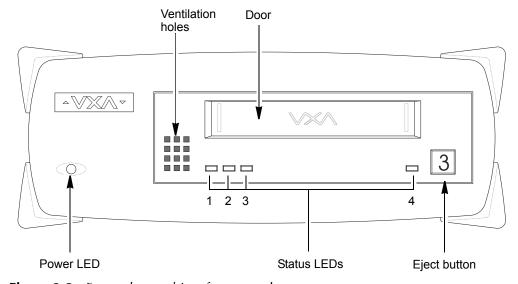
**Figure 3-2** External tape drive: front-panel components
